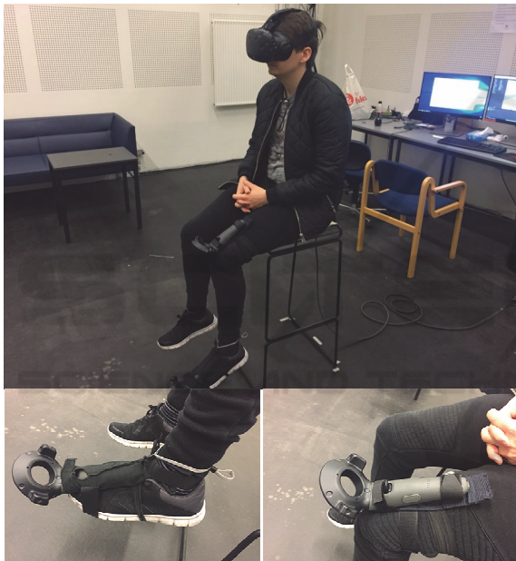
Figure 1: The setup of the experiment. The participant is viewing the game through the HMD while controlling the avatar through the two controllers attached to the left leg.
