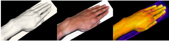
Figure 1: Scanned model contains information from spatial (left), visible (middle) and LWIR spectrum (right).
