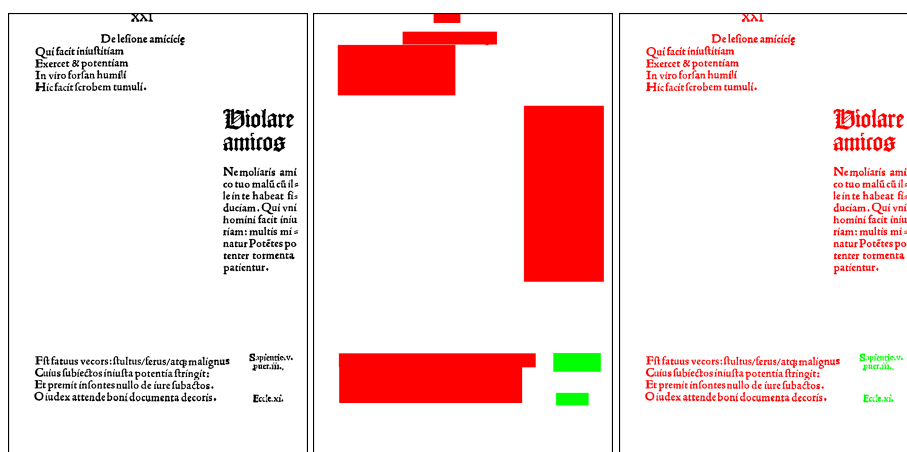
Figure 7: Ground-Truth Generation for Main & Side Body Segregation.
