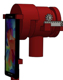
Figure 12: Mechanical prototype showing both the smartphone support and the rack and pinion mate.
