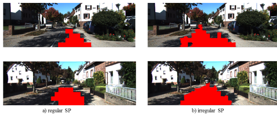
Figure 7: Road segmentation prediction with SP-CNN for two samples based on: a) fixed-size superpixels (Patches), b) irregular superpixels.
