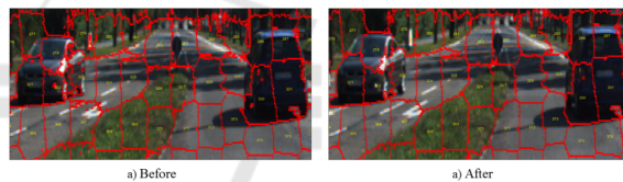
Figure 3: Superpixel segmentation before and after enforce connectivity. It embeds disconnected superpixels into the nearest neighborhood.
