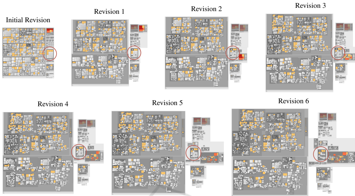
Figure 5: The evolution of the ElasticSearch software project over six months using EvoCells layouting. Removed nodes remains as ghosts in the layout. A particularly stable module is circled red in each revision.
