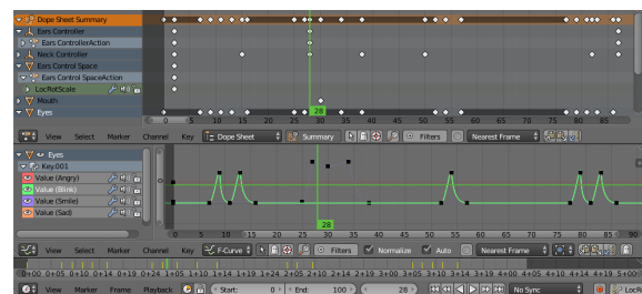
Figure 12: Keyframes animation interface in Blender. The top part shows the dope-sheet and the bottom part the F-curve editor .
