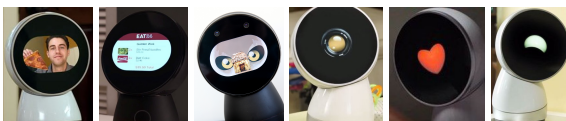
Figure 6: Different functions of Jibo's screen. From left to right, Jibo's screen is used to display the stream of a videoconference, a graphical user interface, an illustration of children's story, an icon indicating the current application, an icon expressing an emotion and a facial expression.
