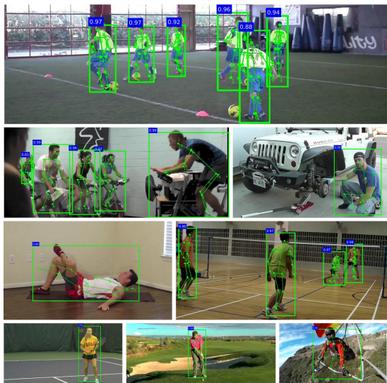
Figure 1: Example pose estimations with the pre-trained network. Samples are taken randomly from the testing set of the MPII Human Pose dataset. The green bounding boxes are the results of person detection and the number on the top-left corner is the probability of a box containing a person.
