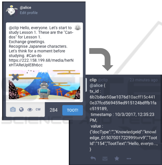
Figure 5: Record of articles in Hyperledger Fabric (Top: posting articles, Bottom: responding to the completion of registration from the clip).
