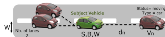
Figure 1: Driving Situation parameters. Subject vehicle speed S , brake status B and wheel information W , the inter-vehicle distance d_n , the relative speed V_n , type and status of the surrounding vehicles, lane width W and number of lanes.
