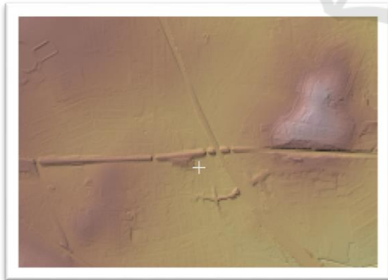
Figure 2: Cuttings and embankments in the EA DTM.
