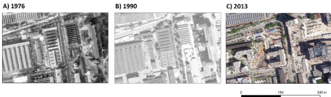
Figure 14: An example of fragments of archival (A, B) and current (C) orthophotomaps in which industrial objects were located and where the analysis of the increased intensity of harmful substances may be performed.
