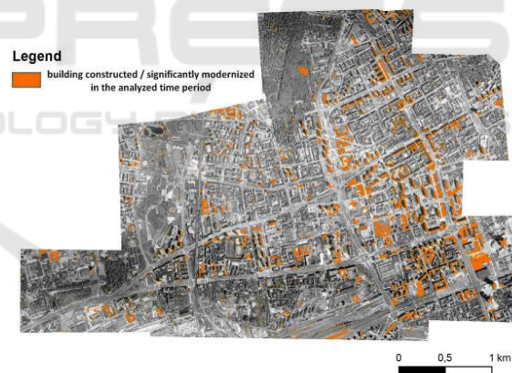
Figure 6: Raster showing constructed and highly modernised buildings within the test site in the period 1976-2013. The orthophotomap of 1982 is shown in the background.
