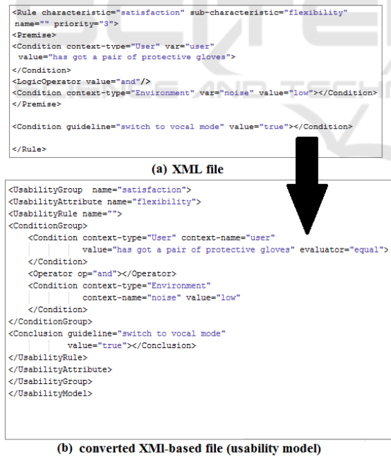
Figure 7: Consistent usability rules: (a) XML file, (b) converted XML-based file.
