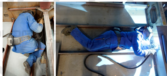
Figure 1: Shipyard welders working in awkward poses.
