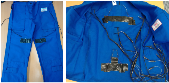
Figure 5: Integration of the tactors into regular workwear.
