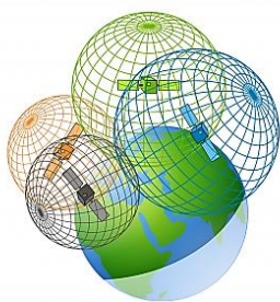
Figure 1: Geometric interpretation of absolute positioning (after http://gisgeography.com/trilateration-triangulation-gps/ ).
