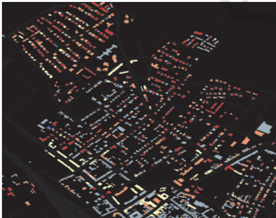
Figure 7: Greenhouse gas emissions per building and year from blue (< 40 kg CO 2 equiv./m 2 a) to red (> 180 kg CO 2 equiv./m 2 a).
