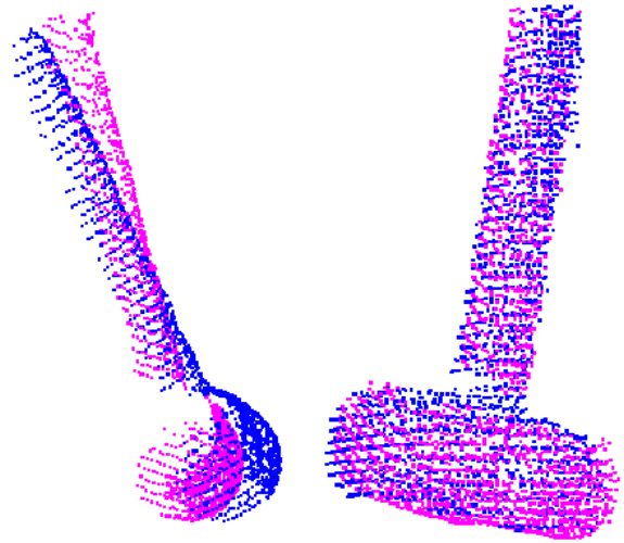
Figure 1: Point cloud of Hammer model before (left) and after(right) submitted from ICP algorithm (Aleotti et al., 2014).
