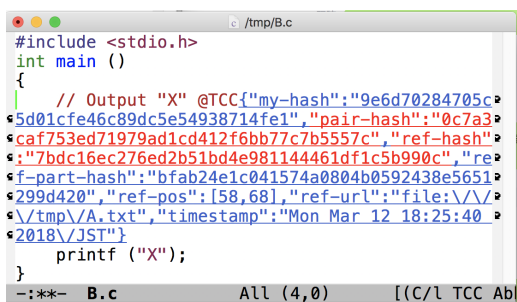
Figure 11: TCC detects the inconsistency between A.txt and B.c.
