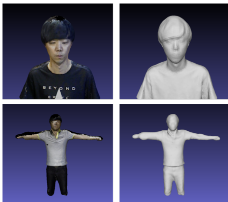
Figure 6: Keyframe pose estimation using 3D registration between subvolumes. Generated texture mapping model(left) and mesh model(right).
