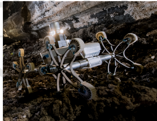
Figure 1: The Asguard V4 rover. A four leg-wheel hybrid robot designed for difficult outdoor environments, equipped with an embedded quad core i7 CPU, a Velodyne LiDAR, Xsens IMU and a 360 degree camera. Additionally the rover can carry payloads of up to 5 kg (e.g. a spectroscope or sampling drill) Image: Robbie Shone, ESA.
