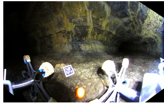
Figure 6: Shows an artificial landmark (magenta colored sphere) placed on a position for which ground truth information was available. The Apriltag in the background was used to distinguish between different landmarks.
