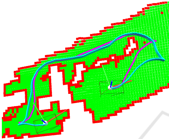
Figure 12: Path planning test in the cave with a lot of obstacles. The cyan trajectory is optimal, the magenta trajectory is a suboptimal solution. The wireframe boxes show the robot's bounding box. The coordinate systems show the start and end pose of the robot.
