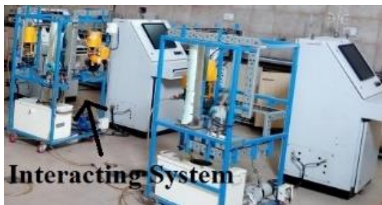
Figure 12: Experimental setup for interacting two tank system.
