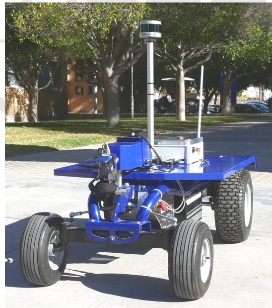
Figure 1: BLUE is a UGV designed to support research in localization and autonomous navigation. Its low-level speed control is based on a Hall effect and a Single-Dimensional Kalman Filter.
