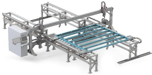
Figure 2: Steel framing machine.
