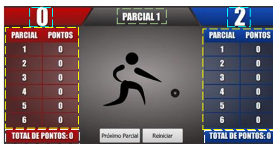
Figure 3: Developed GUI in Portuguese language. Dashed in blue – current score; dashed in green – number of the end being played; dashed in yellow –registry of the score from the six ends; dashed in white – total score.
