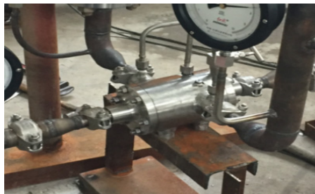
Figure 4: The prototype of the hydraulic turbocharger.
