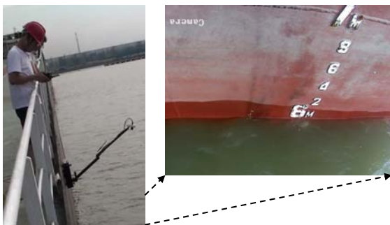
Figure 2: The draft image of bulk carrier An** captured by the climbing robot.
