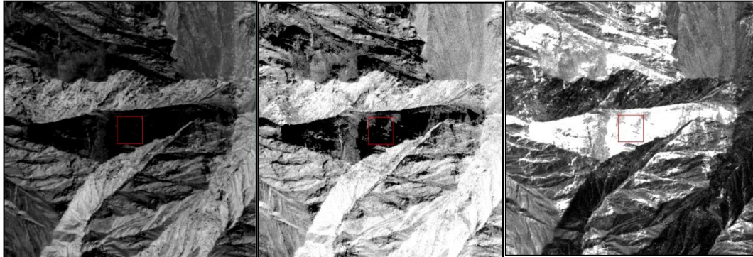
Figure 1: Image contrast of GeoEye-1 before and after data ratio operation (Left: B1; Middle: B3; Right: B1/B3).
