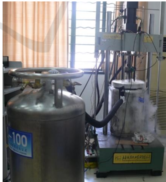
Figure 2. Specimen installed in fatigue machine.
