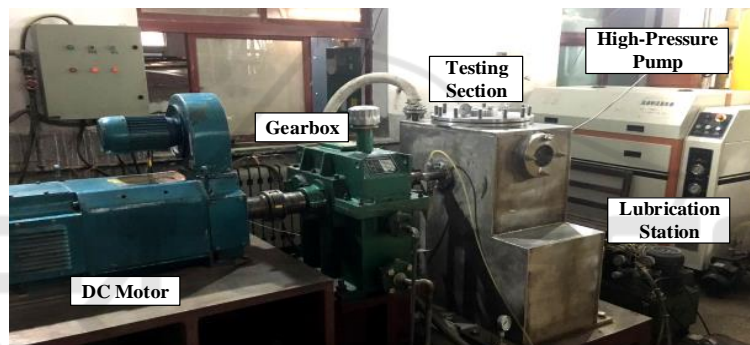
Figure 2. Physical picture of water erosion experiment system.
