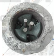
Figure 6 Assembly of mold and mold casing.
