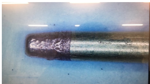
Figure 4 Copper conical tube electrode.
