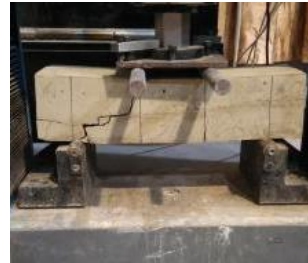
Figure 10. Support point failure.
