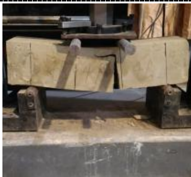
Figure 11. Pressure surface failure.
