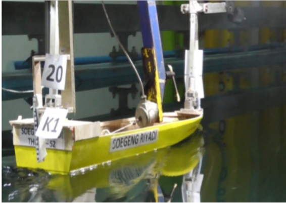
Figure 3: Ship Model of The 31 m Hard-chine Crew Boat Towed at 20 knots ( Fr = 0.62 ).
