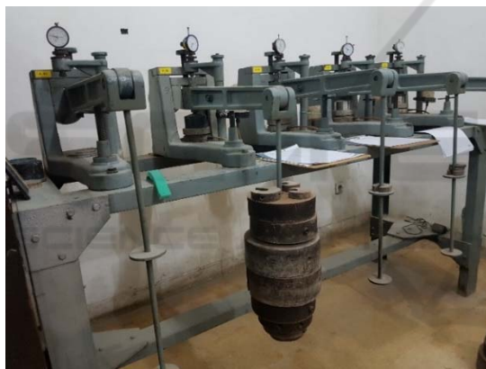
Figure 4: Maximum weight set up to 128 kg (2560 kPa). And not possible to add more weight.
