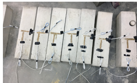
Figure 2: Installation of Strain Gauges on Concrete Specimens.
