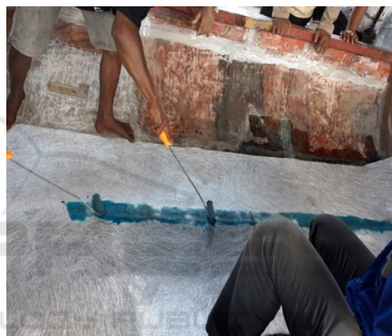
Figure 5: Installation of WR 600 at keel of the boat.
