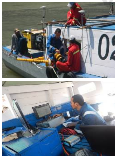
Figure 10: Echo sounder MBES Field Survey.
