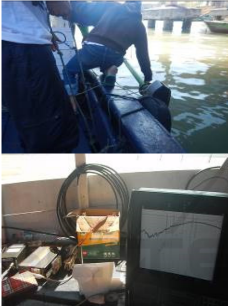
Figure 7: Echo sounder SBES Filed Survey.
