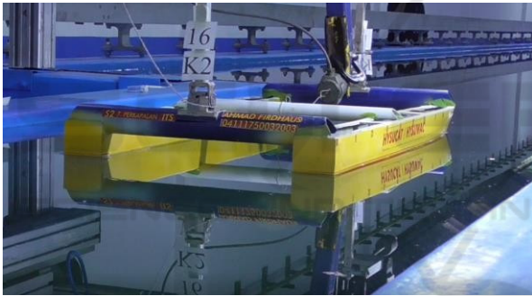
Figure 6: Model 2 of a catamaran with one foil on the bow section of the demihull catamaran before tested on towing tank on 16-knot speed (1.16m/s).
