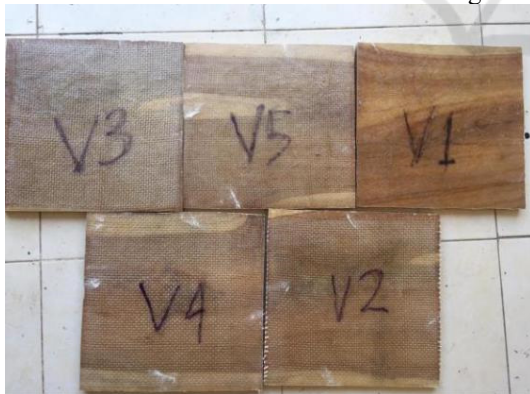
Figure 6: laminated wood with fiberglass.
