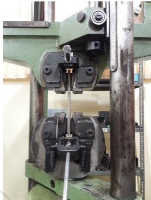
Figure 7: Universal testing machine MFL / UFD 2.0.
