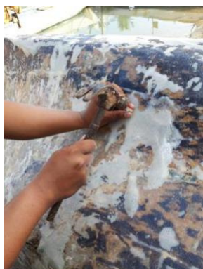
Figure 13: Nailing on the fiberglass layer.
