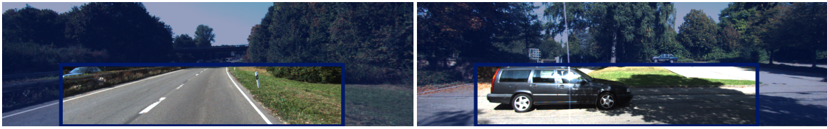
Figure 2: Images from the KITTI Visual Odometry / SLAM benchmark, Sequence 01 (left) and 03 (right). The input images are cropped (thick border) in order for them to contain a large portion of a near planar surface. This assumption is only valid in a subset of the sequences, e.g. the highway of Sequence 01 (left). In many cases occlusions, such as the car in Sequence 03 (right), or the non-planar background surface, is not approximated well by the planar motion model. These situations often occur at road intersections and turns. Image credit: KITTI dataset (Geiger et al., 2012).
