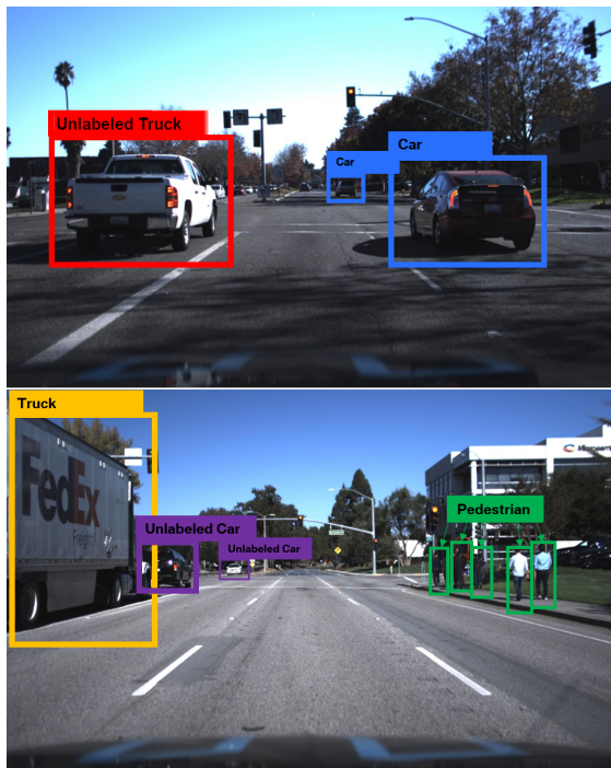
Figure 2: Illustration of used datasets: Top: Sample image from DS1 with labeled cars. Bottom: Sample image from DS2 with labeled pedestrians/trucks and unlabeled cars. The samples are taken from Udacity’s annotated driving dataset by CrowdAI (Udacity, 2017).
