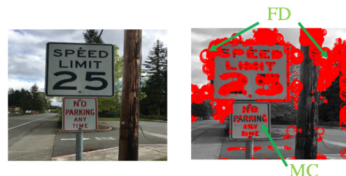
Figure 10: Detection results without contrast normalization (FD) false detections (MC) miss cases.
