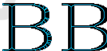
Figure 3: Example of a skeleton without a clipping (left) and with a clipping (right).
