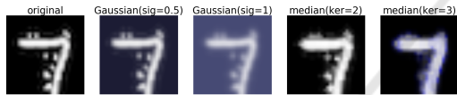
Figure 2: Gaussian & median blur filters at multiple configurations. Both filters are effective to reduce abruptly-occurring pixels in this case.
