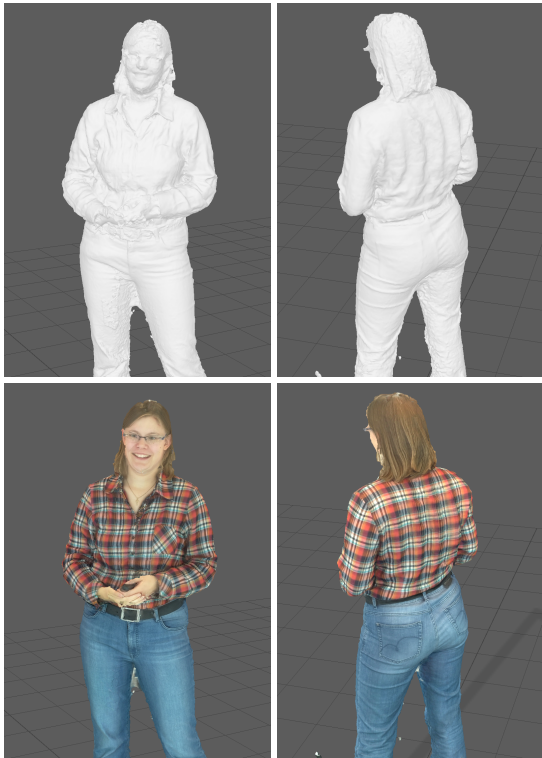
Figure 5: Resulting geometry (top) and fully textured models (bottom) of a typical animated frame of volumetric rendering.
