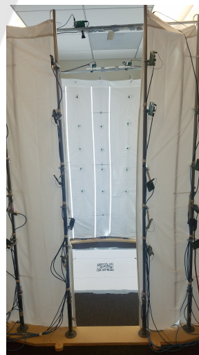
Figure 2: Photogrammetric capture cage consisting of 104 unsynchronized Raspberry Pi cameras; Designed for human body capture and used for volumetric video reconstruction.
