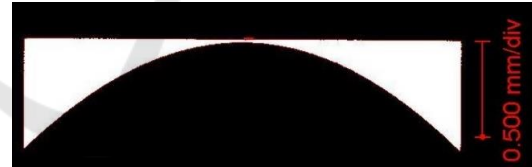
Figure 2: Calculated mask aperture for the fabrication of an 85 \mu\text{m} width cylindrical lens.
