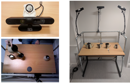
Figure 2: The arrangement of the recording set-up. Top-left image shows the vibration motor attached to an RGB-D camera (Asus Xtion). Right image shows the placement of the cameras in relation to the task table. Bottom-left image shows a colour image taken from the centre camera during a recording.
