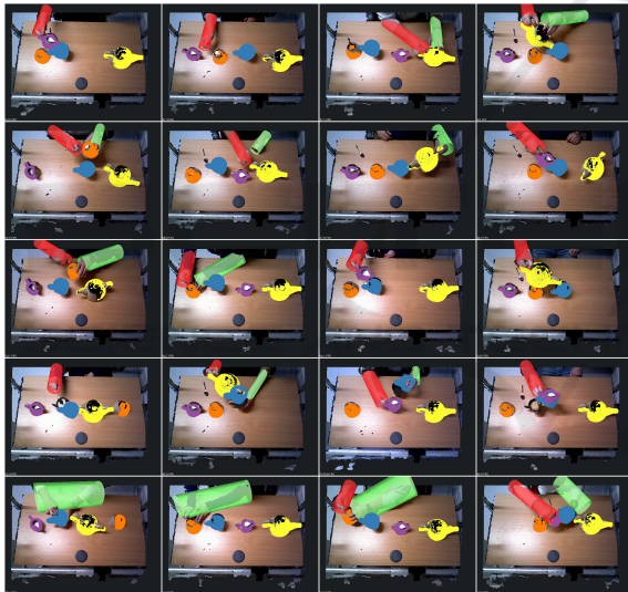
Figure 6: Pose estimation results for different sample recordings. In the first three rows, hand pose and object poses are estimated reliably. In the fourth row, object pose estimation errors are shown. These are due to misalignments of the cup due to changing topology and tracking losses due to complete occlusions. In the final row, arm pose estimation errors are shown. These errors are due to incorrect segmentation of left and right arm clusters when the hands are close together, and incorrect estimation based on inclusion of points from the subject's body.
