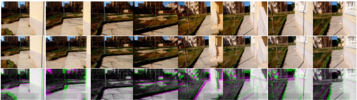
Figure 3: Example of BIDAD-based Outdoor Alignment. The top and the middle rows represent some selected frames from the query sequence and their corresponding frames in the original one, respectively. The bottom row represents the fusion image where the Red & Blue channels in the RGB image are assigned to the query frame, while the Green channel is assigned to its corresponding frame.
