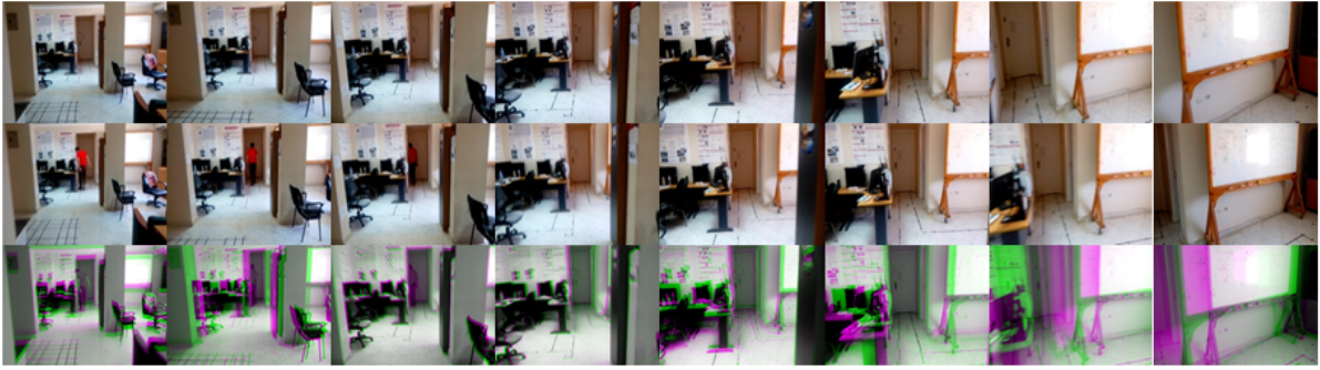
Figure 2: Example of BIDAD-based Indoor Alignment. The top and the middle rows represent some selected frames from the query sequence and their corresponding frames in the original one, respectively. The bottom row represents the fusion image where the Red & Blue channels in the RGB image are assigned to the query frame, while the Green channel is assigned to its corresponding frame.
