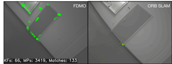
Figure 7: Features matched of FDMO (left) and ORB-SLAM2 (right) in a feature deprived environment (sequence 40 of the Tum_mono dataset).
