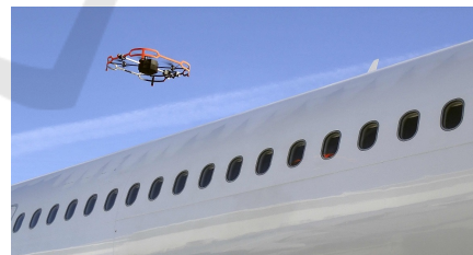
Figure 1: Donecle UAV inspecting an aircraft.
