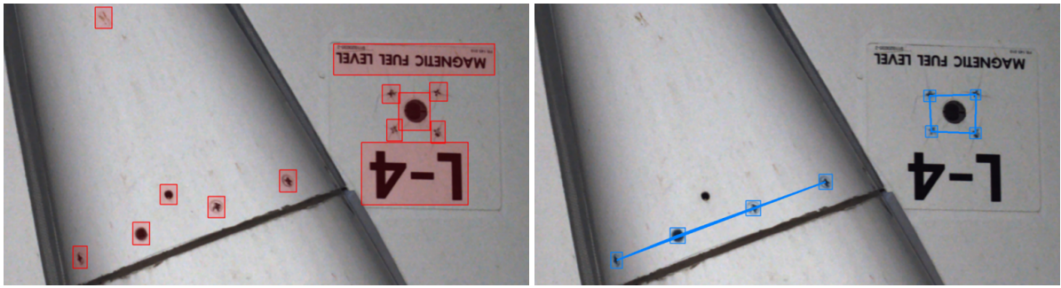
Figure 5: From left to right, detected zones of interest and screw patterns expectation.
